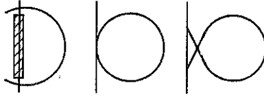
Figure 1. Schematics of the TEXT-U configurations. From left to right, double null, belt limited, equatorial single null.
