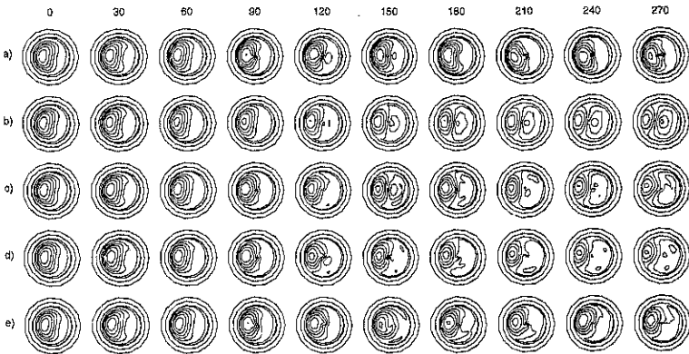
Figure 2: These graphs show the flux surfaces defined by the field in the plane of the instability. Simulation times are in Alfvén times and the simulations are detailed in Table 1.
